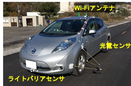
Fig. 1 Pass-by noise levels measurement system
