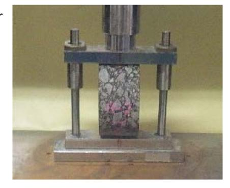
P: maximum load (N), d: thickness of specimen (mm), L: diameter of specimen (mm), x: specimen displacement at maximum load applied (mm)
