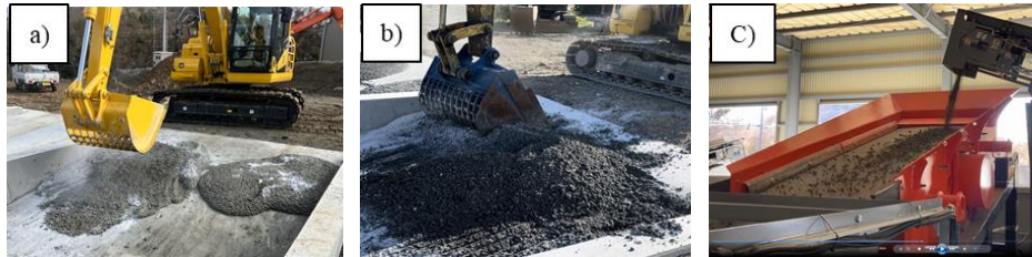
Photo 1 GRA production process: a) Granulating, b) Crushing, c) Sieving
